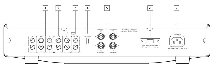
1. Audio inputs (A1-A4) - These inputs are suitable for any 'line level' source equipment such as the audio outputs of CD players, streaming devices such as a Chromecast Audio (RCA Phono to jack cable required) etc.
