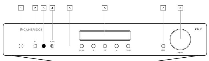
**1.** Power button - Switches the unit between Standby mode (indicated by dim LED) and On (indicated by bright LED). Standby mode is a low power mode where the power consumption is less than 0.5 Watts.
